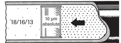
Between 1300 up to (and including) 2500 number of particles equal to or larger than 4 µm(c) per millilitre of fluid.
