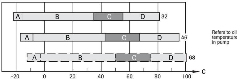
E.g. Hydraulic oil 32: The designation "32" denotes the viscosity is 32 cSt at 40 °C. Lowest start temperature will be -23 °C and highest working temperature 82 °C. Ideal working temperature is 35 - 55 °C.
