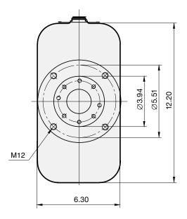
With intermittent operation the gearbox should be filled with 0.13 gal of hypoid oil. Circulation lubrication is required with continuous operation to ensure cooling.
