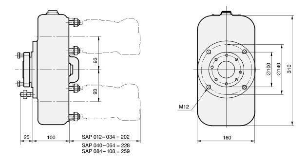
With intermittent operation the gearbox should be filled with 0.5 litres of hypoid oil. Circulation lubrication is required with continuous operation to ensure cooling.
