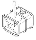
Important by installation! Engine mounted power take-off requires an internal diameter of 64 mm (2.5") on suction hose and connection.
