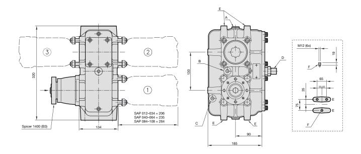
The gearbox must be filled up to the level plug with hypoid oil with intermittent operations.
